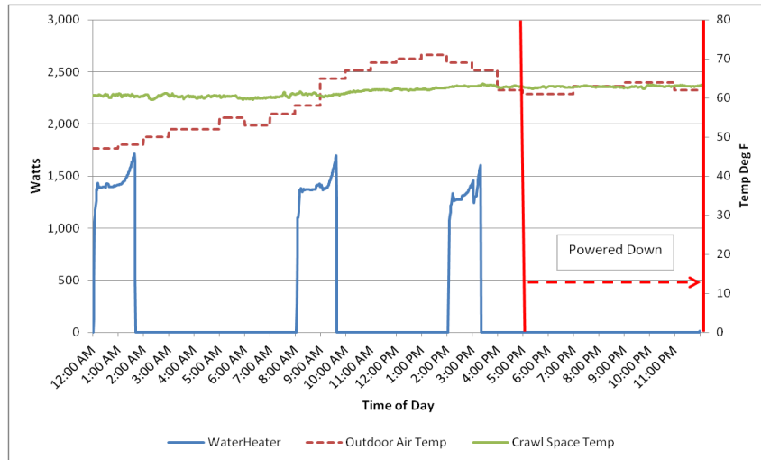
Figure 3.7. Sanden Unitary Oversupply Power Profile: Second DR event (7 hours powered-down), October 22, 2014
