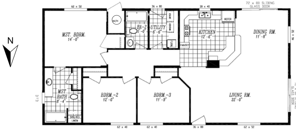
Figure 2. The PNNL Lab Homes consist of two manufactured homes with this identical floor plan set up side by side with the same solar orientation at PNNL’s Richland campus in eastern Washington state.
