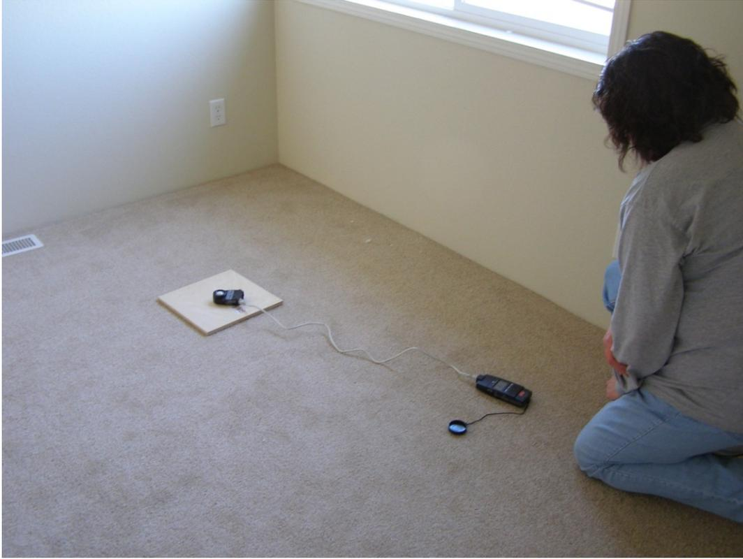
**Figure F.3.** Recording Horizontal Floor-Level Light Level Measurements
