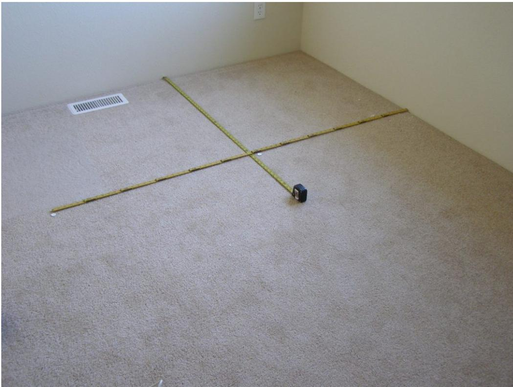
**Figure F.2.** Layout of Horizontal Floor-Level Light Level Measurements
