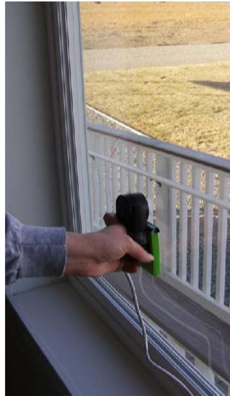
**Figure F.4.** Recording Vertical Light Level Transmittance Measurements Inside
