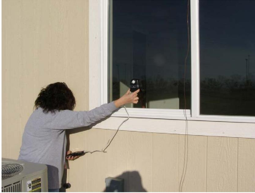
**Figure F.5.** Recording Vertical Light Level Transmittance Measurements Outside
