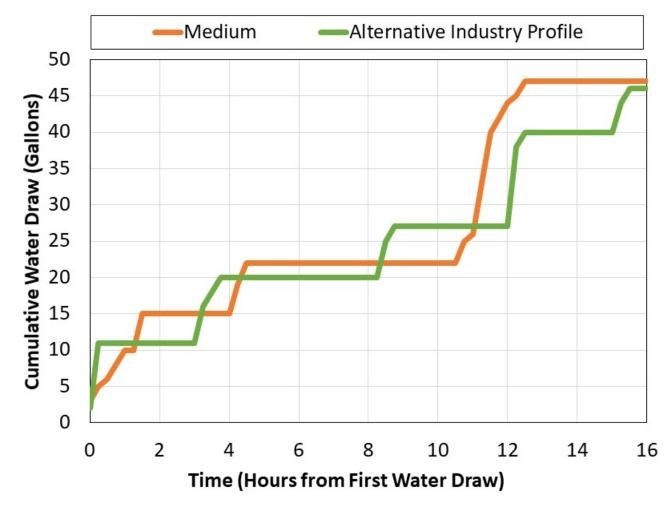
Alternative Profile shown is 3-Occupant Profile from Appendix E of Heat Pump Water Heater Model Validation Study. The two field-based profiles have comparable total daily hot water consumption. The alternative profile consists of 5 time intervals with hot water draws more evenly distributed throughout the day.
