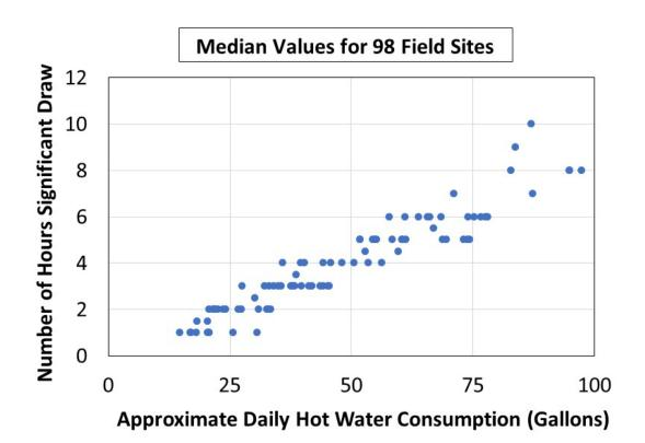
As shown in figure, lower total daily consumption corresponds with fewer hours with a significant hot water draw (i.e. 5+ gallons), and higher total daily consumption corresponds with more significant draw hours.
